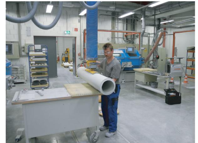
▲ Handling of tube type material
