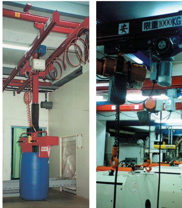
▲ Chemical Tank Handling ▲ Mould Changing System
