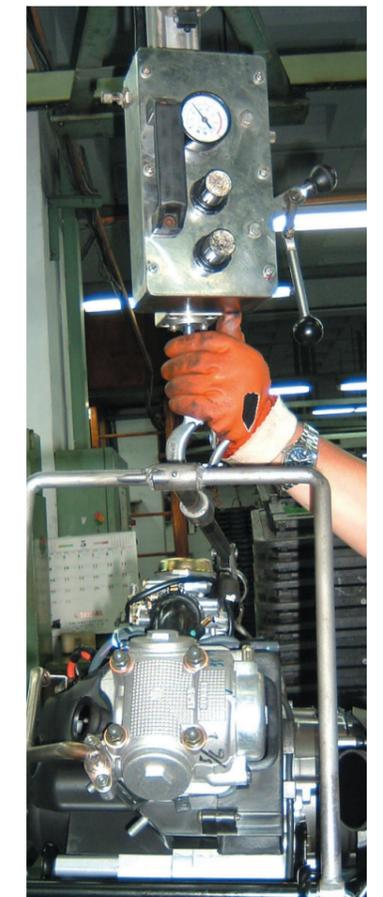
▲ Balance Hanger for Engine Assembly
