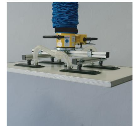
Fourfold suction foot with adjustable pads on main and cross beams
