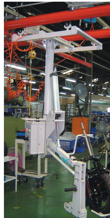
▲ Manipulator for Motorbike Front Wheel Fork Production
