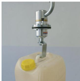
Canister gripper with balancer valve
