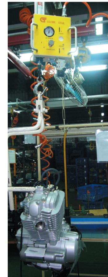
▲ Balance Hanger for Engine Assembly
