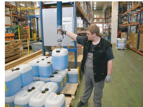
▲ Handling of canisters with mechanical gripper
