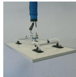
Fourfold suction foot with adjustable suction pads
