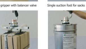
Double suction foot with adjustable suction pads on
