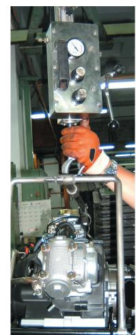
▲ Balance Hanger for **Engine Assembly**
