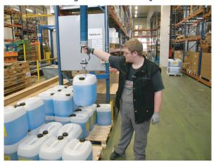
▲ Handling of canisters with mechanical gripper
